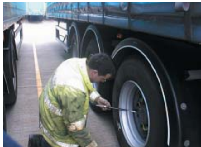
The tyre, interface between vehicle and road. Frequent checks of tyre tread and pressure are vital to ensure vehicle safety. Photo: Michelin
