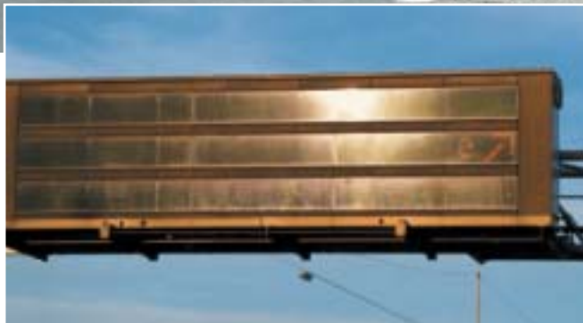
Front screens cause phantom light effects that seriously impair panel readability. Photo: Swarco
